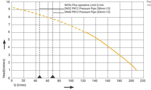
Max. horizontal lenght of pressure pipe incl. 2 elbows and a swing-type check valve 1 1/4"
