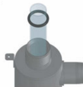
Fig. 6 - Quartz Sleeve Installation
